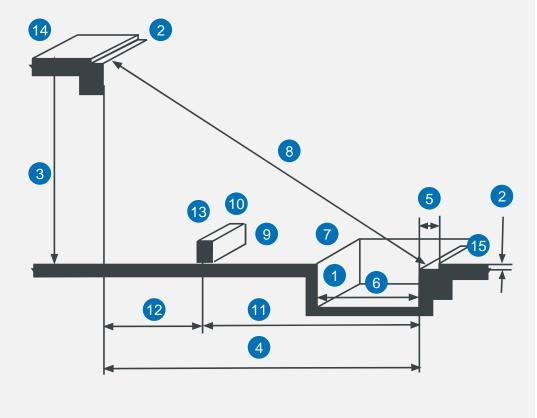
You should ensure that the following measurements are taken prior to installation of the escalator. The dimensions should be checked against the contract-specific KONE layout
